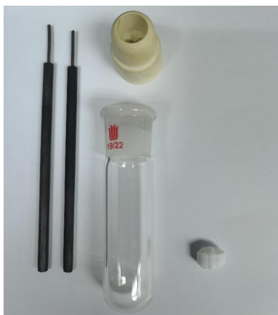
Figure S1. Materials used to make the tube-type electrolytic cell
