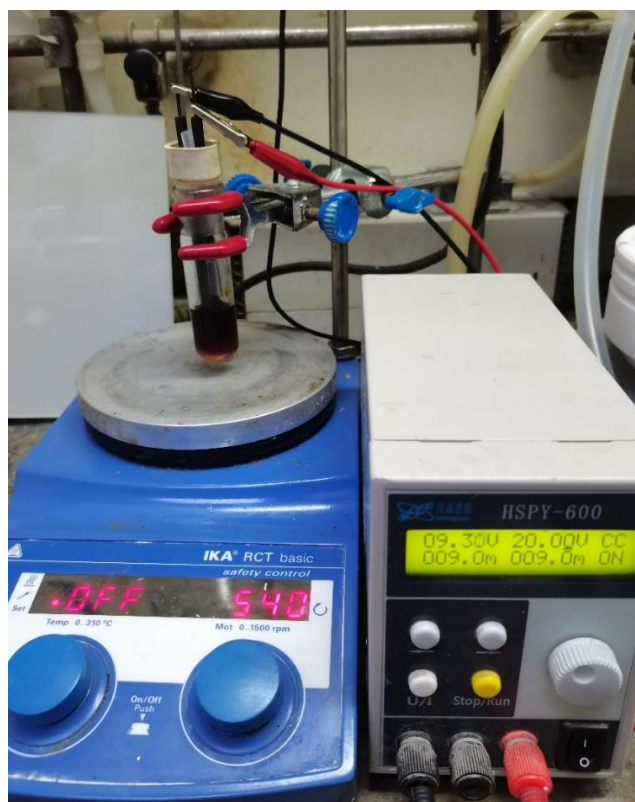
Figure S2. Power supply used in the electrolyze process
