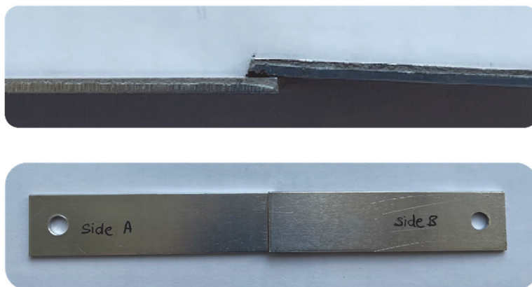
Figure S16. Exemplary picture of DoxL 40 /PCL4MP 60 to showcase the methodology of preparing samples for lap shear experiments.
