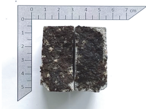
Figure S35. Image of fracture patterns of glued concrete stones using DoxL 40 /PCL4MP 60 as adhesive and cured under saltwater conditions at 70 °C for 1 day (a), 40 °C for 4 days (b), 30 °C for 7 days (c) and 23 °C for 14 days (d). Ruler was displayed with as a reference.
