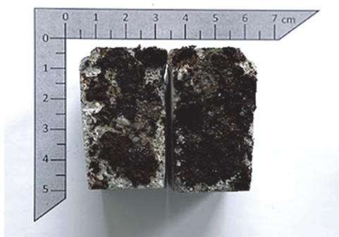
a Underwater Curing 70 °C, 1d
