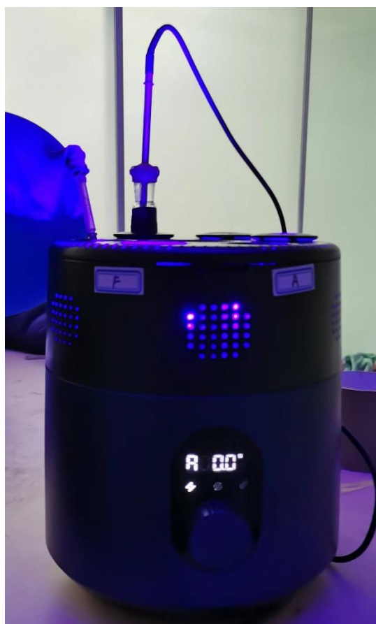
Figure S4. Reaction set-up for irradiation with UV/Green/Blue LED.
