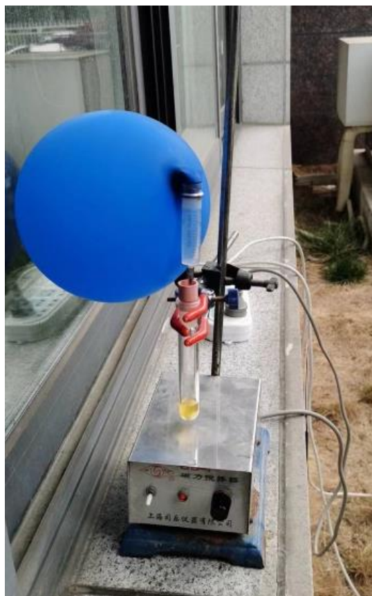
Figure S3. Reaction set-up for irradiation with Sunlight
