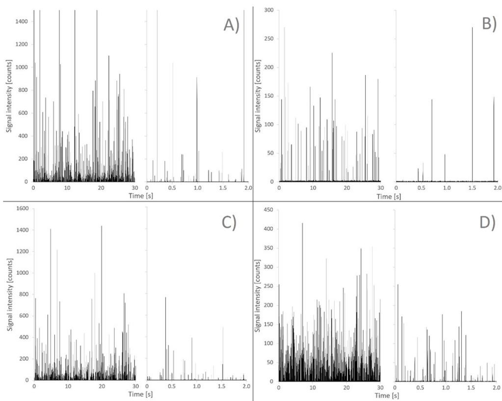
**Fig. SI-1.** Time scans of  $^{80}\text{Se}$  in samples: A) SeNPs after enzymatic procedure ( $1.61 \times 10^8$  particles/L, 1,000-fold dilution), B) SeNPs after mechanical procedure ( $1.46 \times 10^7$  particles/L, 10,000-fold dilution), C) yeast Y-B after enzymatic procedure ( $1.48 \times 10^8$  particles/L, 10,000-fold dilution), D) yeast Y-B after mechanical procedure ( $1.86 \times 10^8$  particles/L, 10,000-fold dilution).
