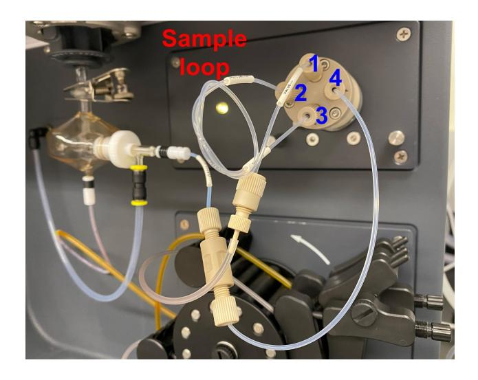
**Fig. S1.** SV4 system with sample loop and the four ports (1 - 4) used for SDA-ICP-OES. See main text and Fig. 2 for additional details.
