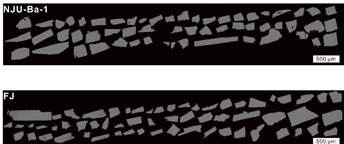
Figure S1. Backscattered electron-imaging result for NJU-Ba-1 and FJ barite. NJU-Ba-1 barite contains small amounts of tiny calcite inclusions, while FJ is nearly pure barite mineral with minimal inclusions.
