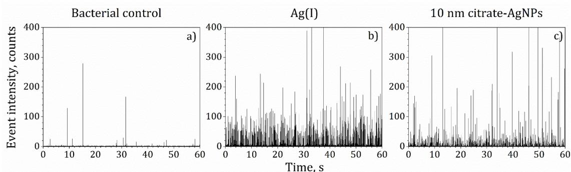
**Figure S4.** Time scans of SC-ICP-MS for *E. coli* bacteria: a) bacterial control, b) bacteria exposed to Ag(I) ( $Y_c = 1$  count;  $Y_{C,N} = 12$  events) and c) bacteria exposed to 10 nm AgNPs ( $Y_c = 1$  count;  $Y_{C,N} = 12$  events). Instrument: Agilent 8900 ICP-MS.
