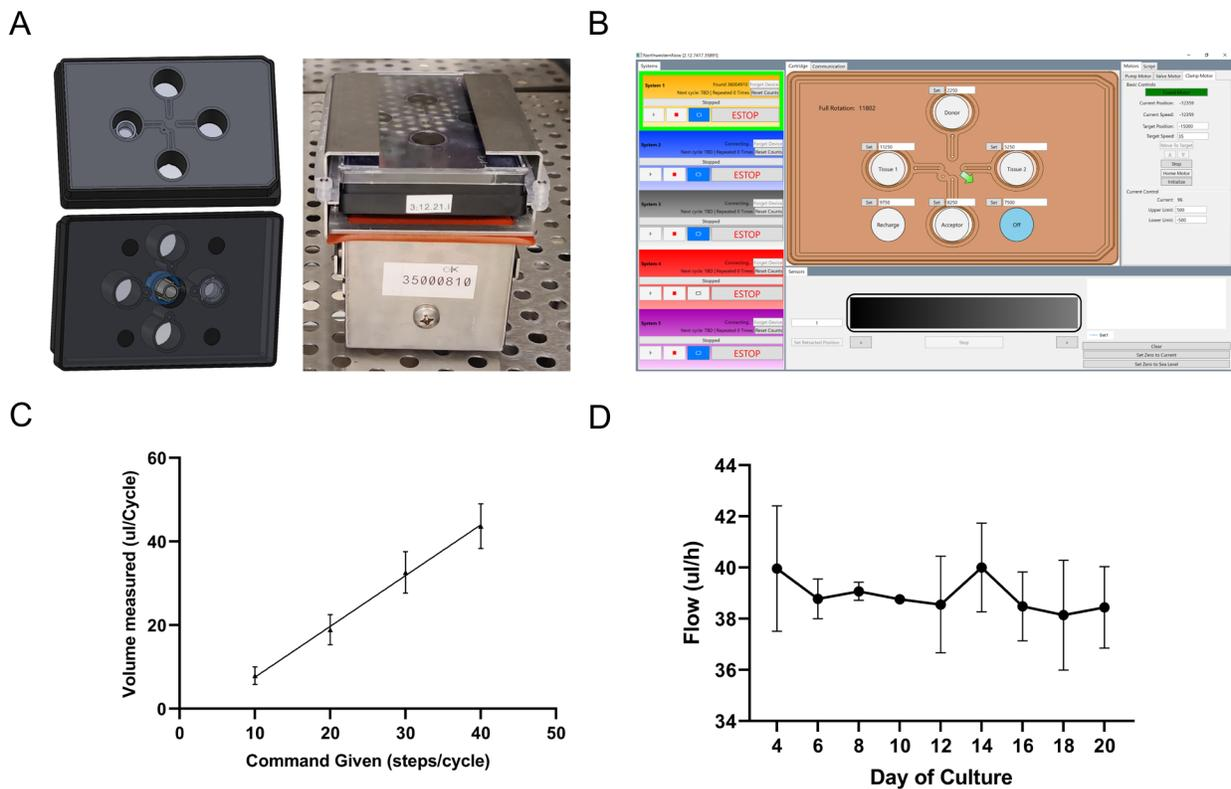
**Fig. S1** 2UP prototype. A. Basic design of the 2UP LATTICE culture plates (left) and engaged with the base station (right). B. Custom 2UP software gives the operator control over the different motors of the base station. This can be done manually or by writing executable scripts that describe each individual step. C. 2UP pump equation ( $n=21$ ) D. Fluid flow during long term culture of 2UP platform.
