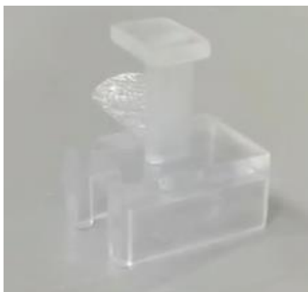
Figure S6-1 A little piece of polyethylene film is stuck between the gel loading module and the anchor module when put them together to make block gel.
