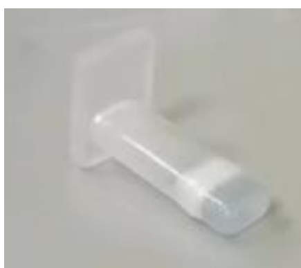
Figure S6-2 A little piece of parafilm is applied to the gel loading module as demonstrated.
