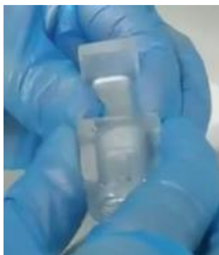
Figure S6-4 Hold them at a slight tilt angle when gently separating them after electroelution is completed.
