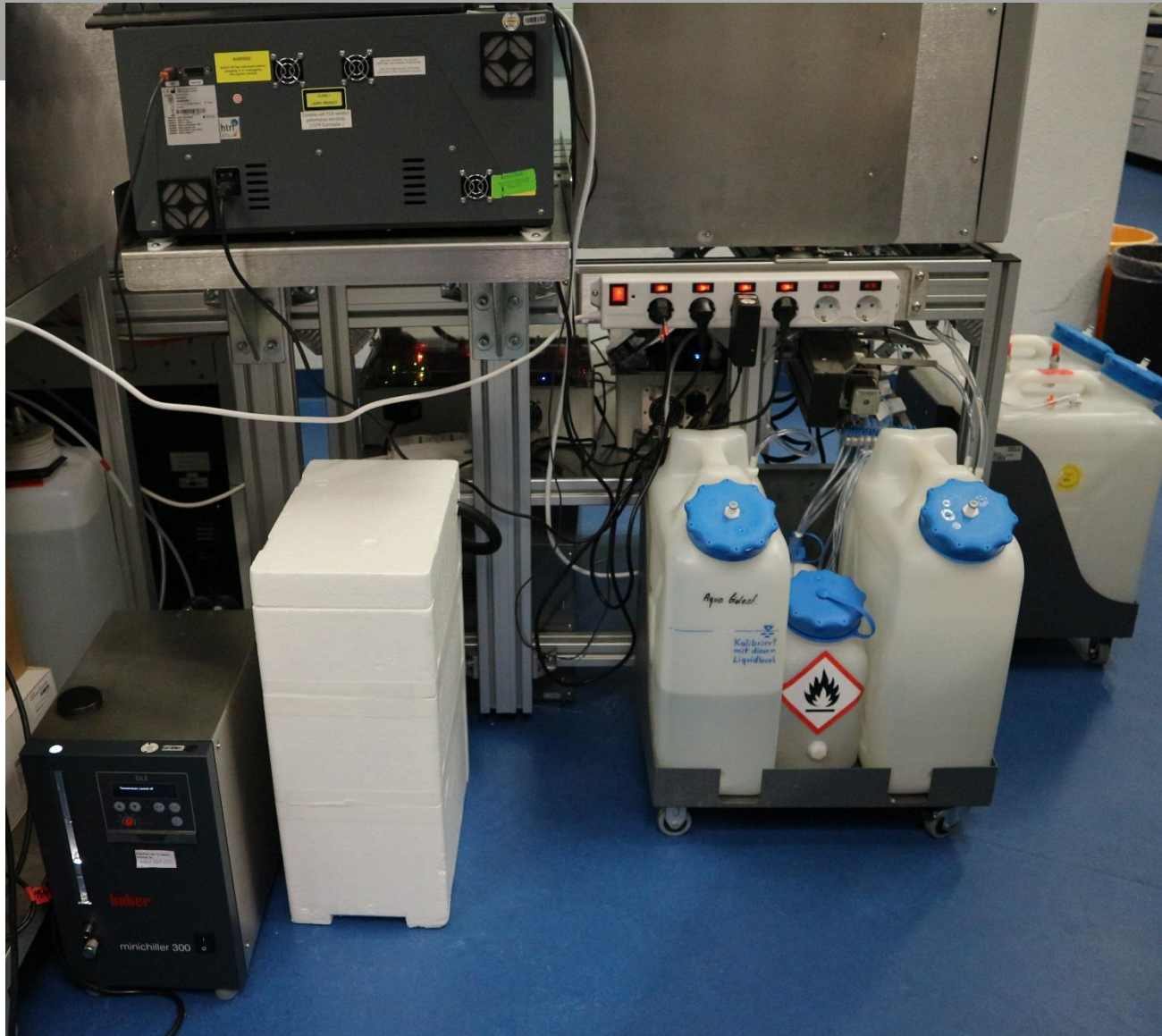
Figure S 15: The liquid handling setup from the back. The white styrofoam box holds the container with the cooling liquid used for the 384-needle cooling operation. Next to the white box is the used cooling device (Huber, Germany) for the cooling of the cooling liquid. Above the cooling setup is the plate reader (Tecan, Switzerland), seen from the back.
