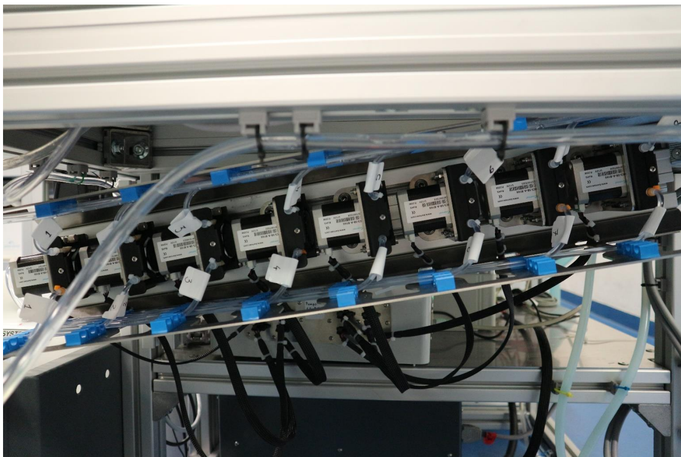
Figure S 17: Solvent pumps for the solvent washing station. Eight peristaltic pumps (Kamoer Fluid Technology, China) were used for this task. To reduce the risk of trapped air the pumps and all tubes for solvent were mounted at an angle.
