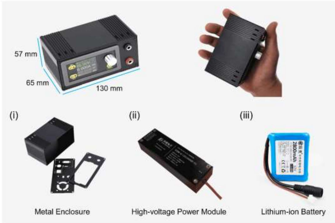
Figure S2. Pictures of a battery-driven voltage source, consisting of a metal enclosure i), a high-voltage power module ii), and a lithium-ion battery iii).
