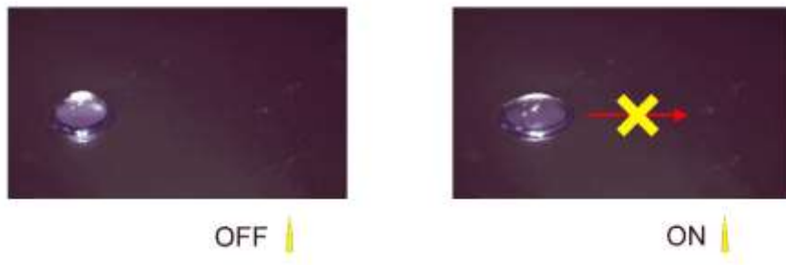
Figure S4. Optical pictures demonstrate that PET film without porous structures cannot actuate the droplet.
