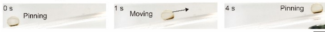
Figure S10. A 10 \mu\text{L} water droplet was successfully transported on a tilted surface ( 8^\circ ) by 1 \mu\text{L} transporter. The scale bar is 2 mm.
