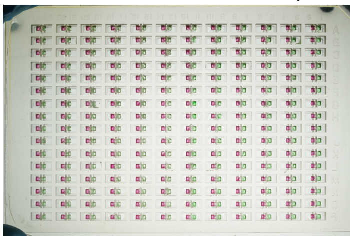
Figure S14. 384-well plate OoCs. Loading of red and green dyed gel solutions into the 384-well plate format OoC devices printed in 1.5 h using the Elegoo Saturn 3 Ultra with a nominal pixel size of 19 \times 24 \mu\text{m}^2 and >58\text{M} pixels. Across three uniquely 3D printed well plates, we observe a 100% yield on fluidic performance of the embedded multi-layer stop valves.
