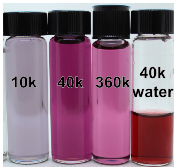
Figure S2. Digital photograph showcasing the different gold colloids in DES, prepared with PVP 10k, 40k and 360k and 40k in water, along with their respective UV-Vis spectra.
