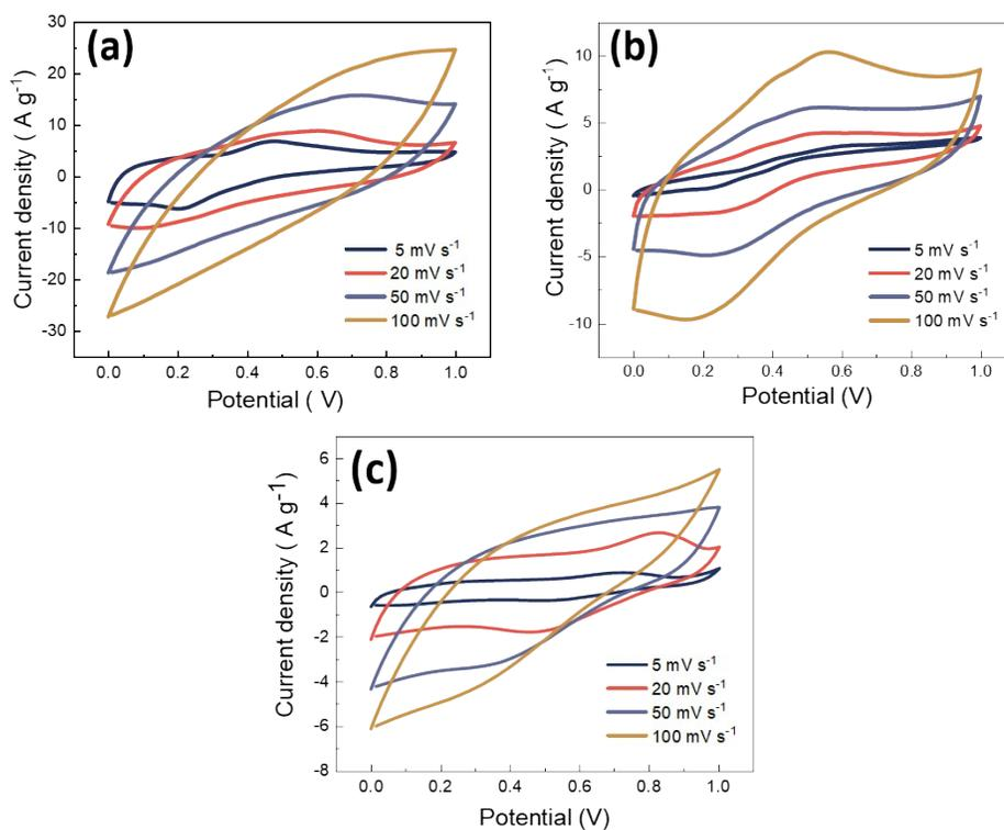
**Figure S2.** Cyclic voltammograms of PANI /MWCNT symmetrical supercapacitor at different scan rates a) PANI/MWCNT (5:1), b) PANI/MWCNT (10:1) and c) PANI/MWCNT (30:1), respectively.
