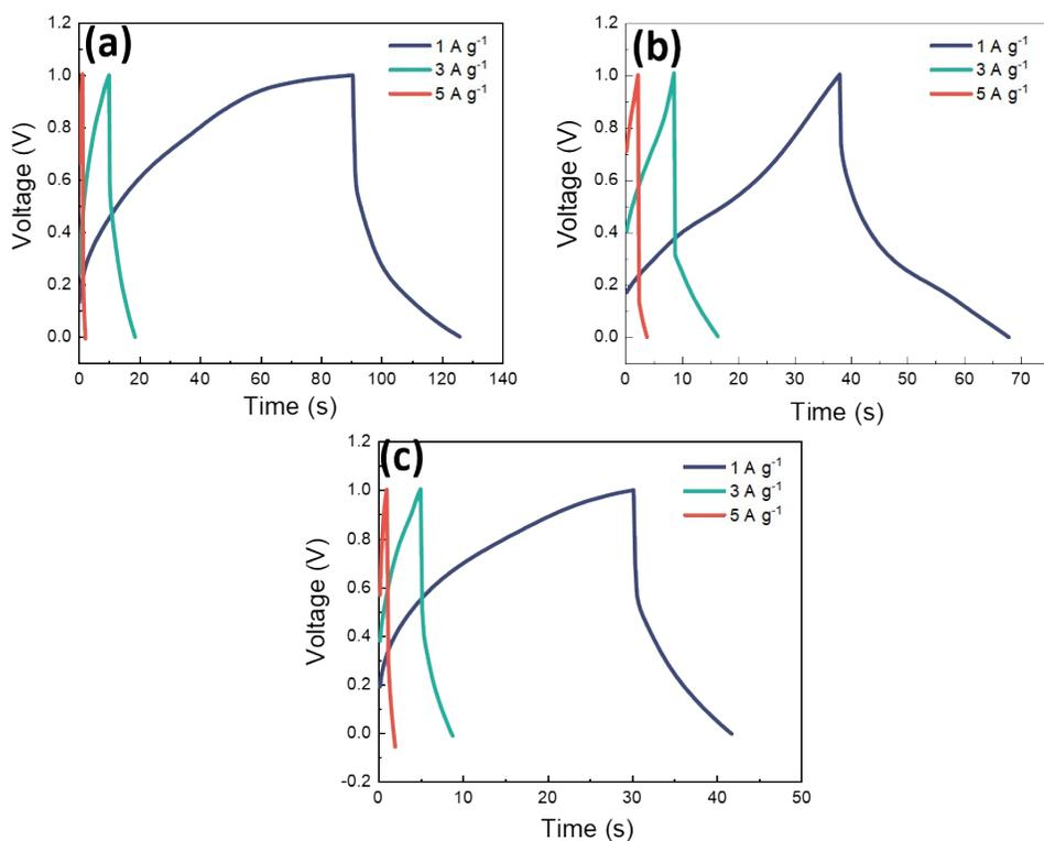
**Figure S1.** GCD curves of (a) PANI/MWCNT (5:1), (b) PANI/MWCNT (10:1), PANI/MWCNT (30:1) at different current densities.
