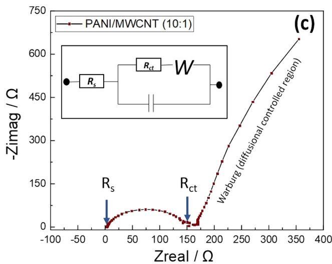
**Figure S3.** Schematic design and (a) picture of a 10 mm diameter Swagelok-type electrochemical cell (b) EIS curve of PANI/MWCNT (10:1) electrode with inset showing Randles equivalent circuit model (c).
