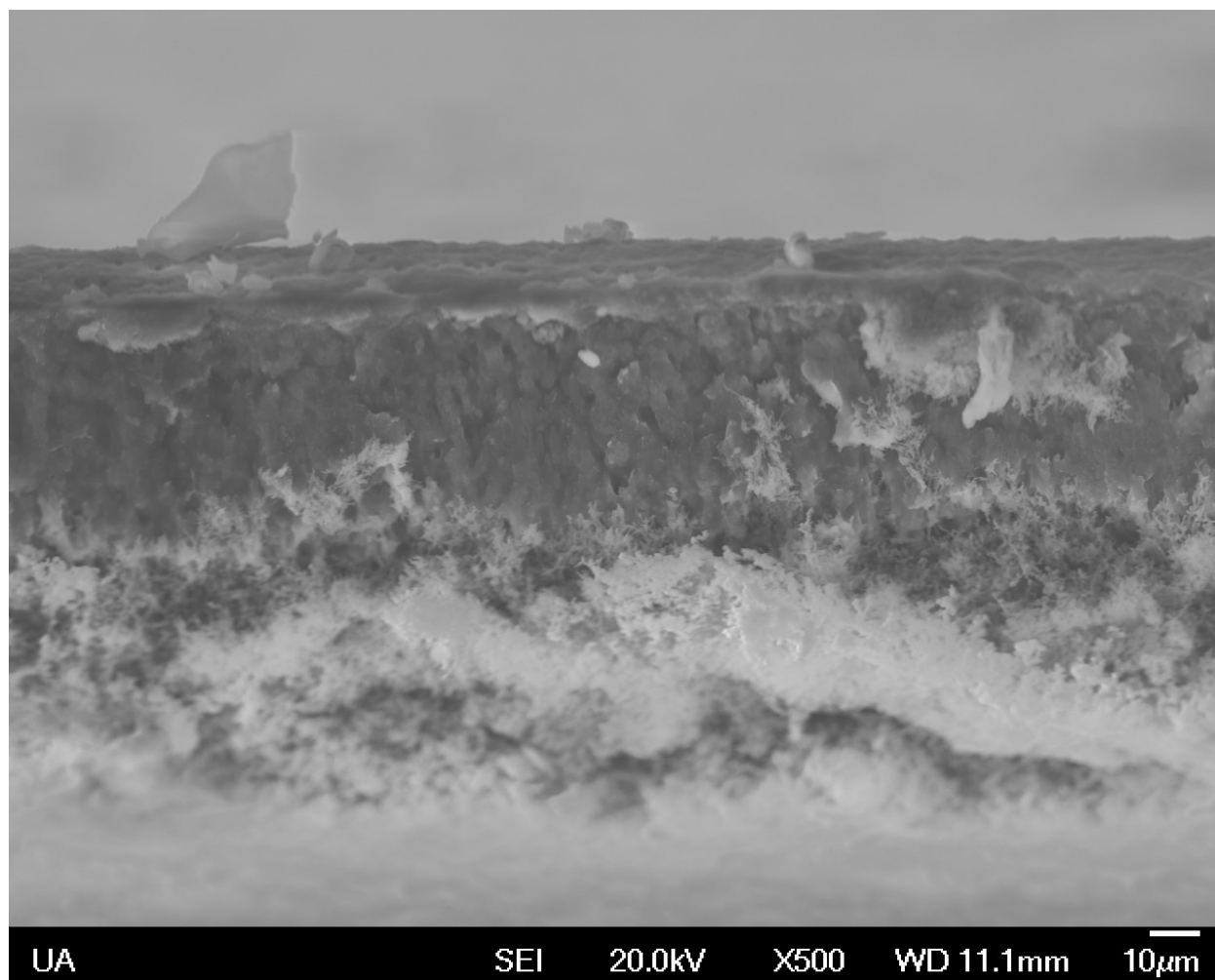
Figure S12. SEM image of [PMDA-2MeAPI(pXy)][Tf 2 N] + [C 4 mim][Tf 2 N] on a Supor ® PES support.
