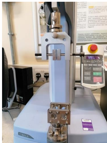
Figure S1: The set up used for peel testing using a Shimadzu EZ-LX universal testing machine with a 500 N tensile jig in the upper position and a peel rolling jig in the lower position.
