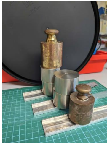
Figure S3: The setup utilized for blocking tests involved placing two strips of Film 3 with adhesive sides facing each other underneath a metal bar. This ensured that the weight applied was evenly distributed across the adhesive-adhesive interface.
