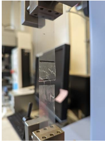
Figure S2: The set up used for shear strength testing using a Shimadzu EZ-LX universal testing machine with with two 500 N tensile jigs.
