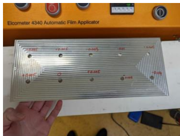
Figure S4: The custom metal template made to hold 8 mm diameter rheometer parallel metal plates. This enabled thin films to be cast over the rheometer plates with a homogeneous thickness. The numbers quoted on the plate is the error between the height of the template and parallel plates in mm.
