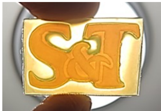
SI Figure 5. Overcured S&T logo printed with DP 10000 CFS
