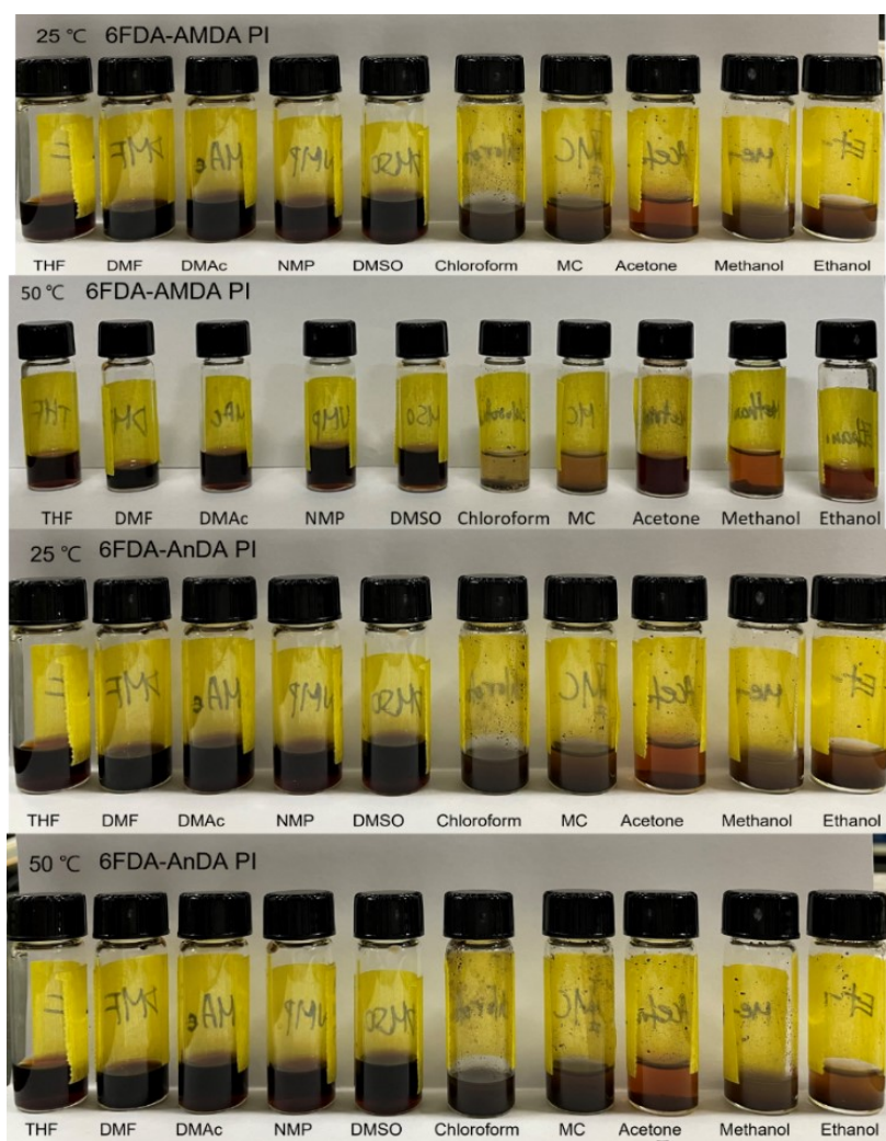
Figure S4. Solutions of 6FDA-AMDA PI and 6FDA-AnDA PI in various solvents.
