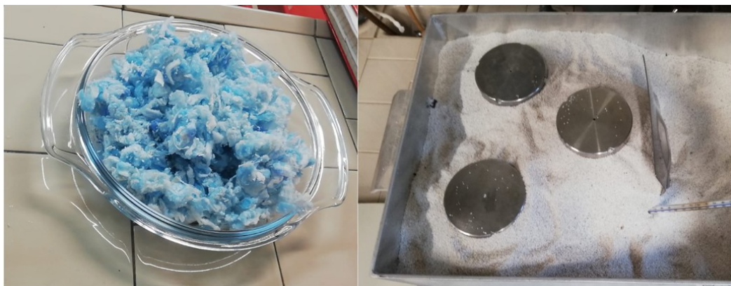
Figure S.1. On the left, the mashed facemasks. On the right panel, the vessels dived in the sand bath during the hydrothermal process.
