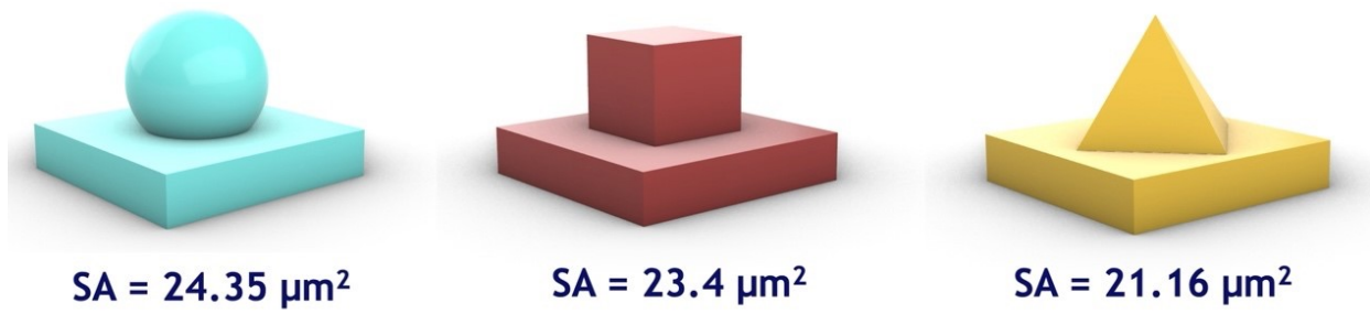
Figure S2. Enhancement in effective contact surface area among various pattern features: microdome, cube and pyramid. The surface area values were calculated using similar pattern height (2.5 \mu\text{m} ) and projected width (2 \mu\text{m} ) by Rhino software version 7.0.
