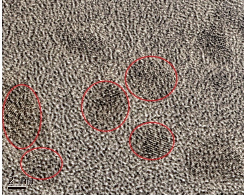
Fig. S8: HRTEM image of CG-MW with few marked particles.
