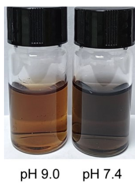
Figure S2 Photograph of FeL_3Mn_3 at pH = 7.4 and 9.0 (in Tris buffer, 0.1 M ).
