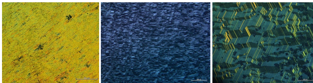
Figure S29. Cross-polarized optical micrographs observed for aligned compounds S6 and O6 . Alignment was achieved by unidirectional flow of molten compound into a 2- \mu\text{m} -thick cell. Left: S6 at 135 °C, middle: O6 at 130 °C, right: O6 at 30 °C. The kinks in the right image, combined with XRD data, suggest a monoclinic crystal structure with a \sim 5.55 nm, b \sim 1.75 nm and \beta \sim 60^\circ .
