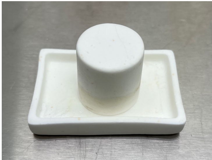
Fig. S12 A picture of the crucible and the lid which covers the powder and the film.
