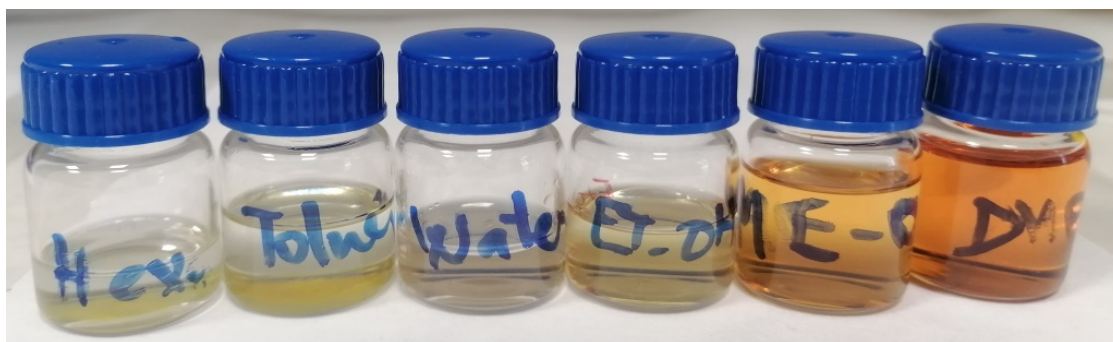
Figure. S1 Solubility of the complex (\text{CH}_3)_2\text{NH}_2[\text{Fe}(\text{phen})\text{Cl}_4] in some selected solvents.
