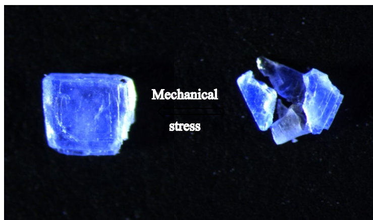
Fig. S9 Fractures of Form II crystal upon application of a mechanical stress under UV light.
