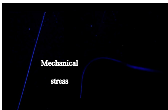
Fig. S7 Screenshots of reversible elastic bending test of Form I crystal under mechanical stress applied through a pair of tweezers under 254 nm UV light.
