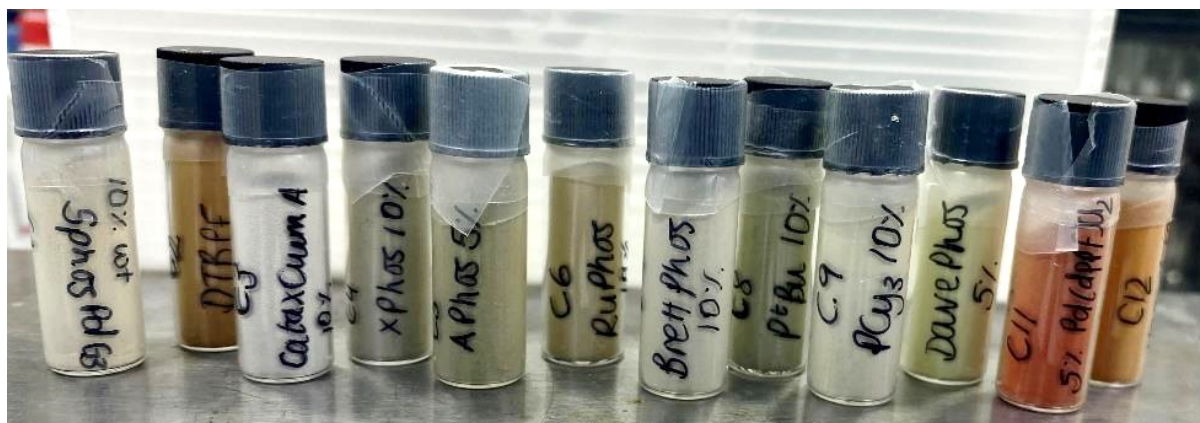
Figure S7: A schematic detailing the procedure used to make the Pd-coated ChemBeads and a photograph of the ChemBeads prepared for the Suzuki-Miyaura screening kit.
