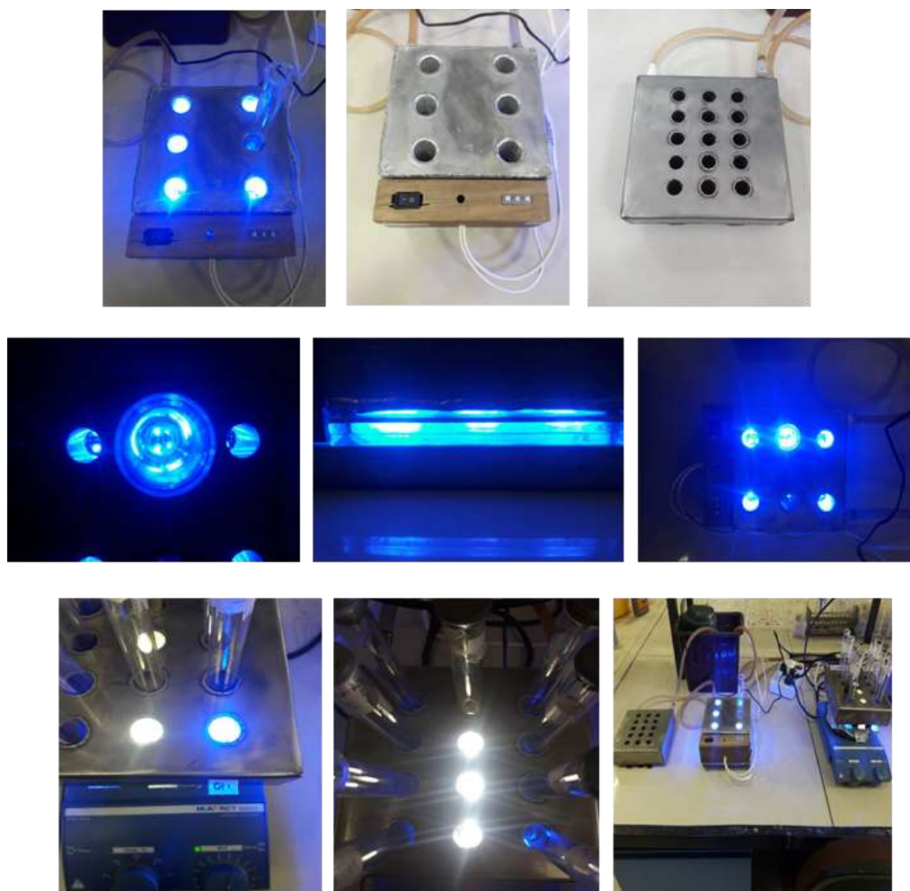
Figure S1. Novel LEDs setup to display high photon offer to the reaction medium
