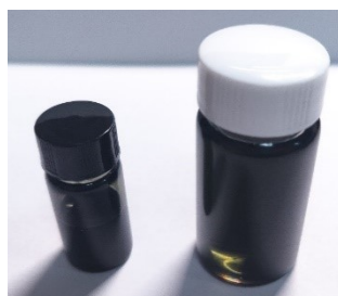
Figure S1. Digital image of \text{Ti}_3\text{C}_2\text{T}_x dispersed in NMP (left) and \text{Ti}_3\text{C}_2\text{T}_x DMAc dispersion at room temperature for 3 months (right).
