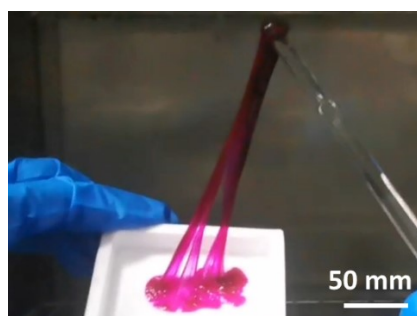
Fig. S25 Photographs demonstrating the flow state of SHPU-WNS at 100 °C. As shown, SHPU-WNS had adhered to the polytetrafluoroethylene mold at 100 °C, suggesting that it had lost the mechanical robustness.
