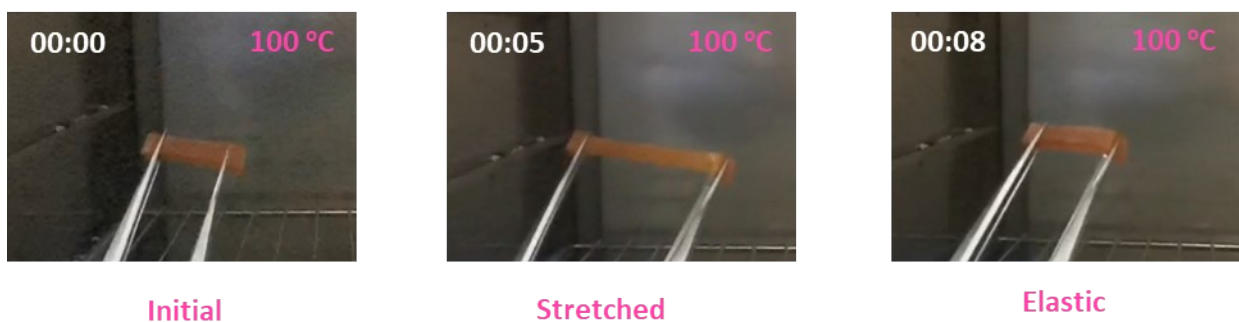
Fig. S24 Photographs of SHPU-SNS-0.3 reversibly stretched at 100 °C. As shown, SHPU-SNS-0.3 could be subjected to reversible large-strain stretching at high temperature, which indicated a high operating temperature for SHPU-SNS-0.3.
