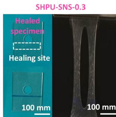
Fig. S23 Photographs of self-healed SHPU-SNS-0.3 specimen that could tolerate puncture and be stretched to 8 times its original length.
