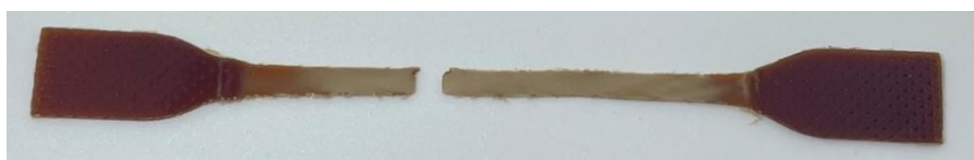
Figure S18. The real picture of tensile fractured dual-nanophase PLA.
