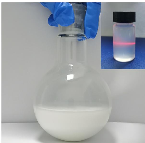
Figure S1 Product of m-LDH prepared by our new method. Inset: Highly dispersed m-LDH with a clear Tyndall effect.
