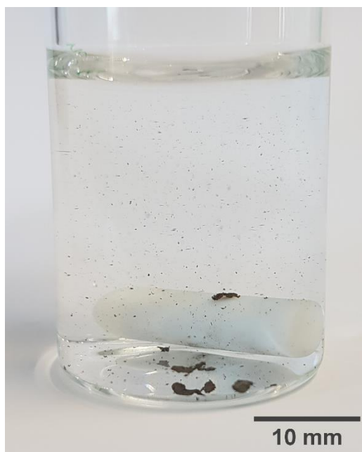
Figure S1. Picture of agglomerated silver nanoparticles in the reacted MGS-Ag(I) system without PVP.
