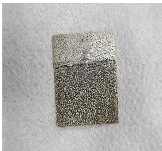
Fig. S5 Digital image of Ni foam as a current collector and drop casted G-ZCO sample as active electrode material.
