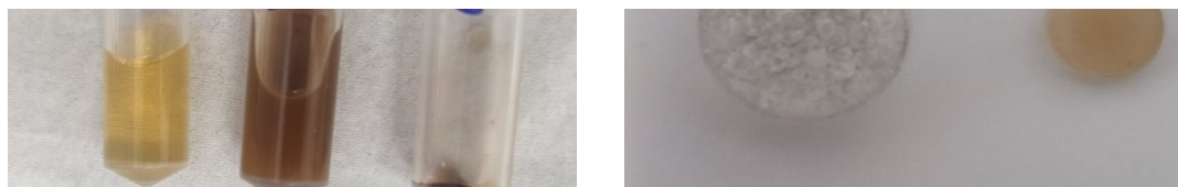
Figure S3 optical image of produced PdNP fractions, B. optical image of hydrated(left) and dehydrated(right) PdNP hydrogel pellet catalyst.
