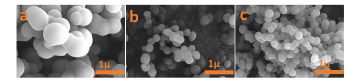
Figure S1: The FESEM images of (a) CX0.01, (b) CX0.05 and (c) CX0.1 at a scale of  $1\mu m$ , after the stability test.
