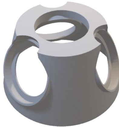
Figure S2: 3D-printed custom chamber for taking pictures of the LFIA strips with the same light conditions, prior assembly of the LEDs.
