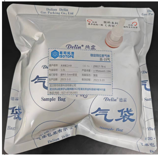
Fig. 25. The ^{15}\text{N}_2 bag for isotope labeling tests.
