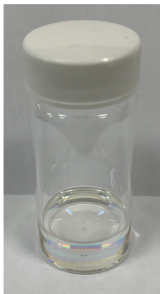
Fig. S9 Photos of (a) the orange solution obtained by washing the cell electrodes before charge-discharge processes using the 5 mL of carbon disulphide and (b) the colorless solution obtained by washing the cell electrodes after charge-discharge processes. The 5 mL of carbon disulfide was used for the washing.
