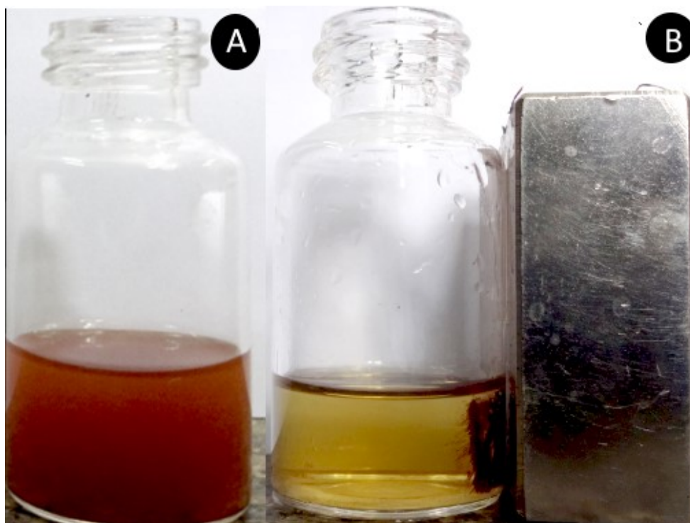
Fig. S2. Images of magnetic recovery A) before the reaction, B) after the reaction.
