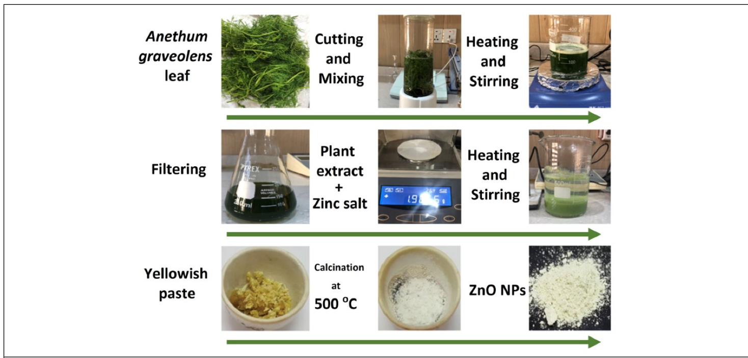
Fig.S1: Graphical demonstration of ZnO NPs formation process utilizing Anethum graveolens leaf extract and zinc acetate dehydrate
