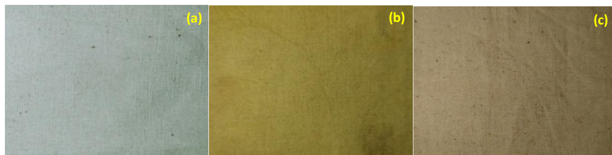
Fig. S22 Photographs of (a) neat cotton fabric, (b) benzoxazine coated cotton fabric and (c) cured cotton fabric
