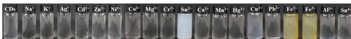
Visual recognition of metal ions (0.5 × 10 -3 M) with the probe N, B-CDs (0.4 mg mL -1 ) in the aqueous medium.
