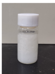
Figure S6. Photographs of the toluene-water emulsion stabilized by 50 mg ZIF-8( photograph was taken after standing for 3 weeks).
