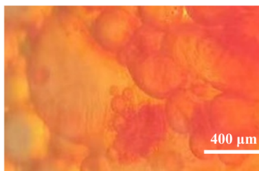
Figure S4. Optical microscope images of the 40 mg ZIF-8 stabilized Pickering emulsion with a water-to-toluene ratio of 3:2 and the emulsion stained with Rhodamine B and methyl red.
