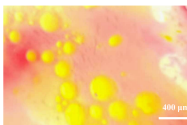
Figure S13. Optical microscope images of water (3 mL)-toluene (2 mL) emulsion stabilized by 50 mg ZIF-8 after the fifth catalytic run.
