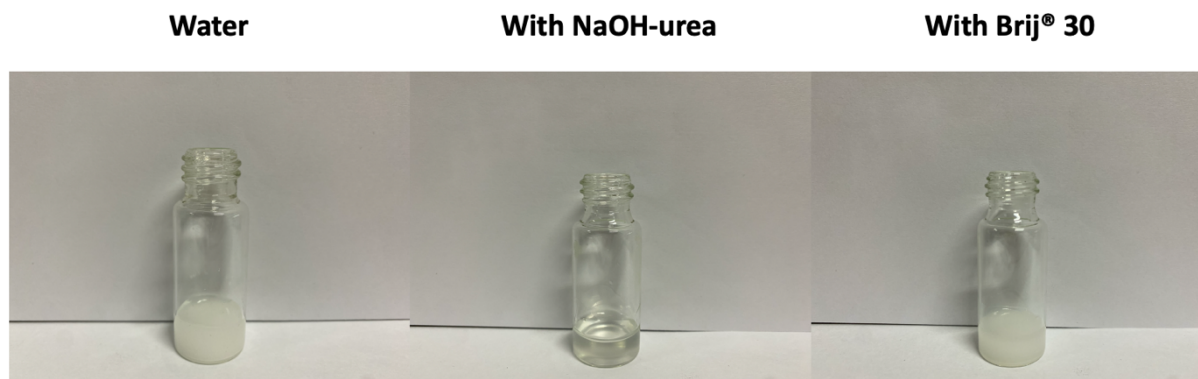
Fig. S1 Homogeneous dissolution of starch in water facilitated by the addition of NaOH-urea and a surfactant (Brij® 30)
