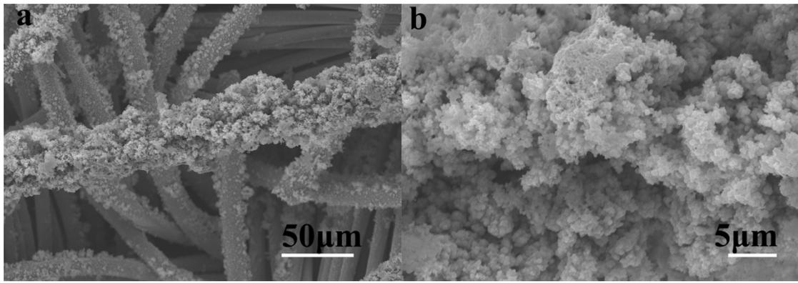
**Figure S4.** Electrodeposition at 50°C.
