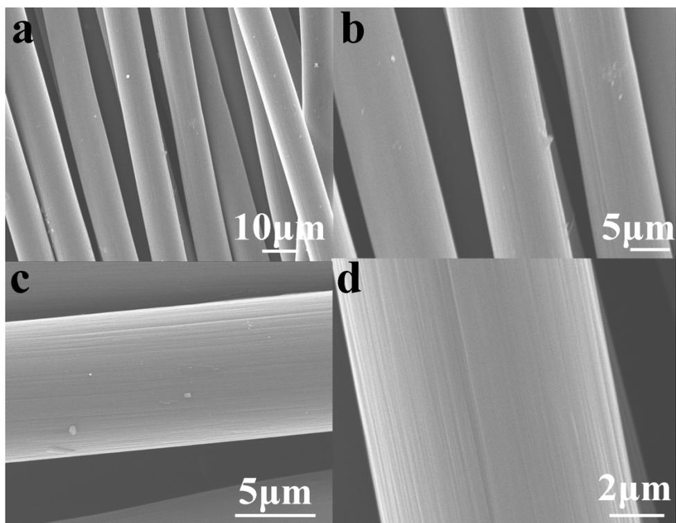
**Figure S1.** SEM of Carbon Cloth.
