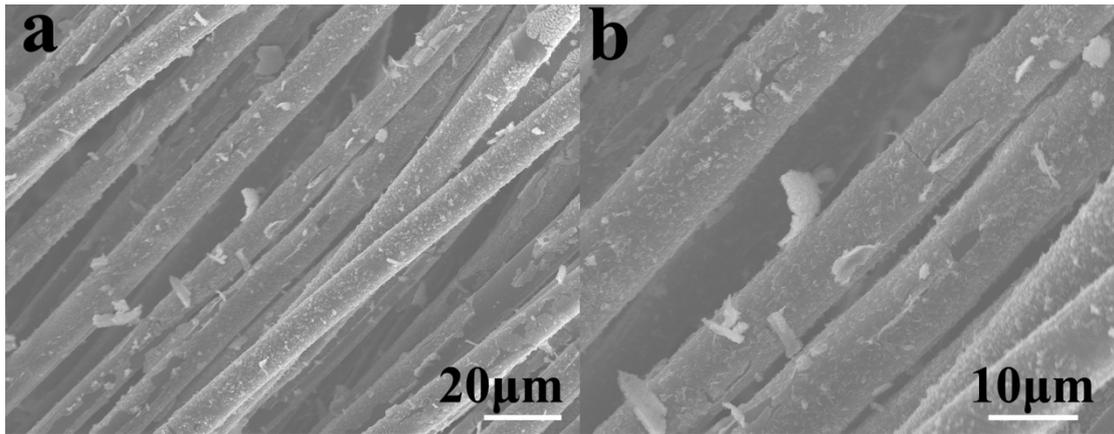
**Figure S7.** SEM of the NiCoSe<sub>2</sub>@CC after the cycle.
