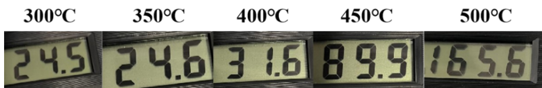
Fig. S4 Resistance value of FTO conductive glass annealed at different Al-reduction temperatures.
