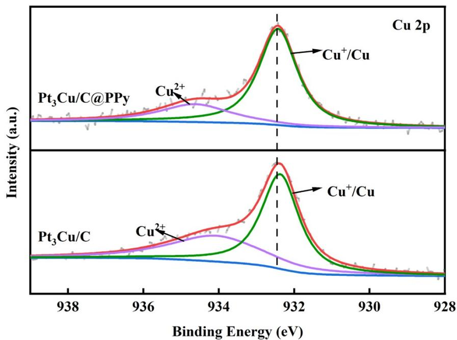
Fig. S1. Cu 2p XPS peak plot of Pt<sub>3</sub>Cu/C@PPy and Pt<sub>3</sub>Cu/C
