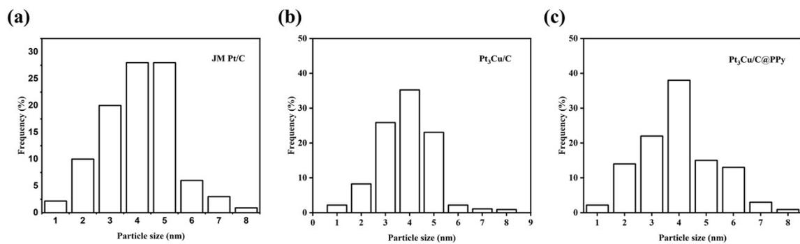
**Fig. S4. Particle-size histograms of (a) JM Pt/C, (b) Pt<sub>3</sub>Cu/C and (c) Pt<sub>3</sub>Cu/C@0.4-PPy after ADT test**
