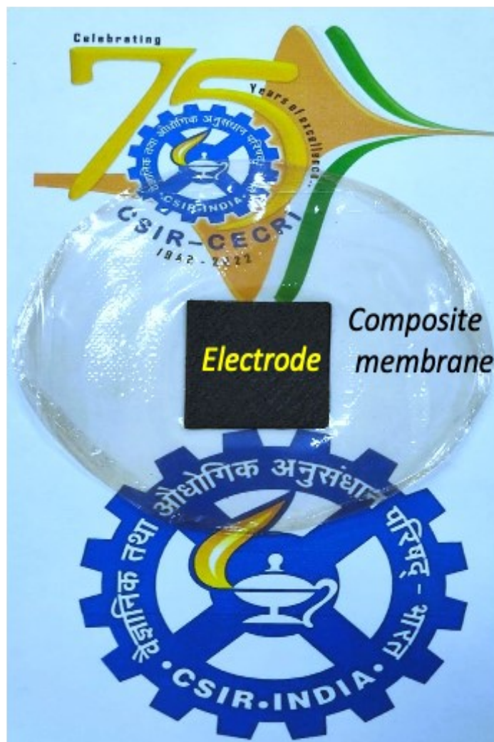
Figure S19: Snapshot of s PEEK/Cu-PMA-0.5 wt.% composite membrane-based MEA.
